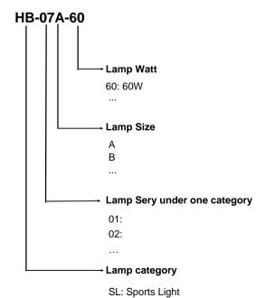
HB: Highbay RL: Road Light WW: Wall Washer LL: Linear Light Neon: LED strip light
