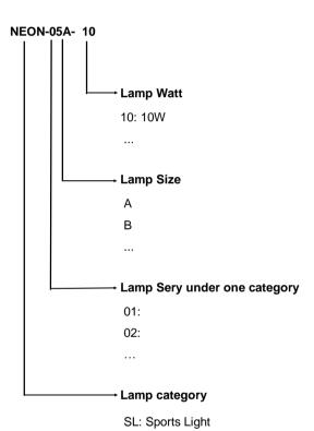
HB: Highbay RL: Road Light WW: Wall Washer LL: Linear Light Neon: LED strip light
